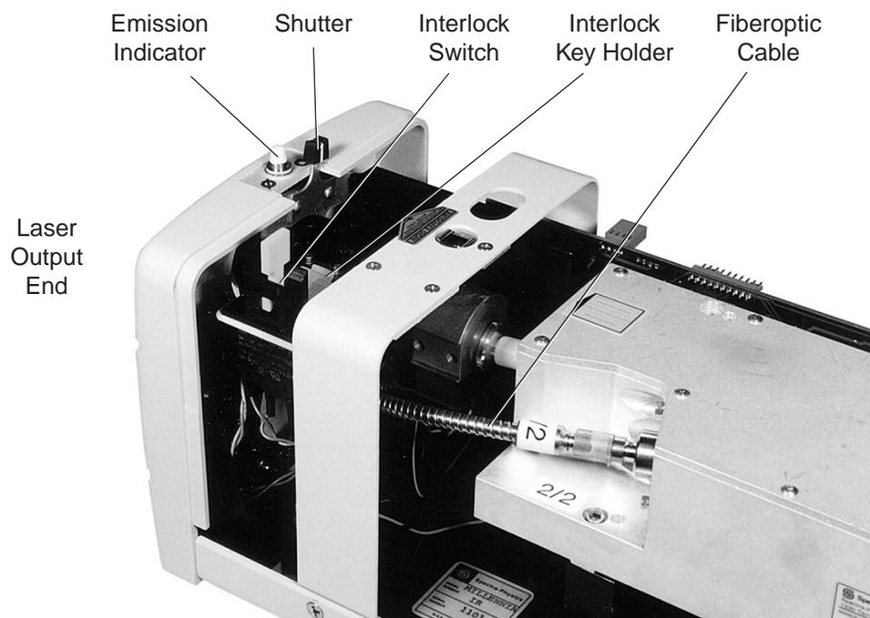
**Figure 2-4: Laser Head Emission Indicator, Shutter and Safety Interlock**
