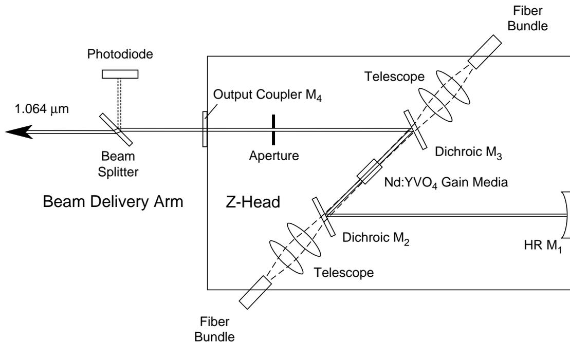
**Figure 3-9: Schematic of the Millennium IR Laser Head**
