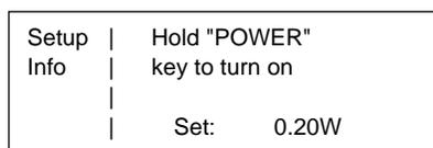
Press and hold in the LASER POWER button until the laser starts. When the button is pressed, the LASER EMISSION light flashes for a few seconds. Then, when laser emission occurs, it stops flashing and remains on, and the emission indicator on the laser head turns on to indicate radiation is present.
