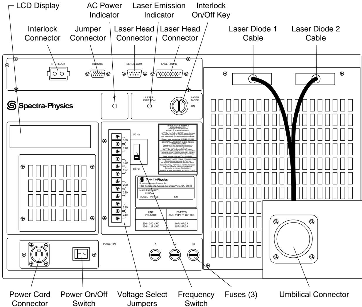
**Figure 4-4: The T40 Power Supply Control Panel**
