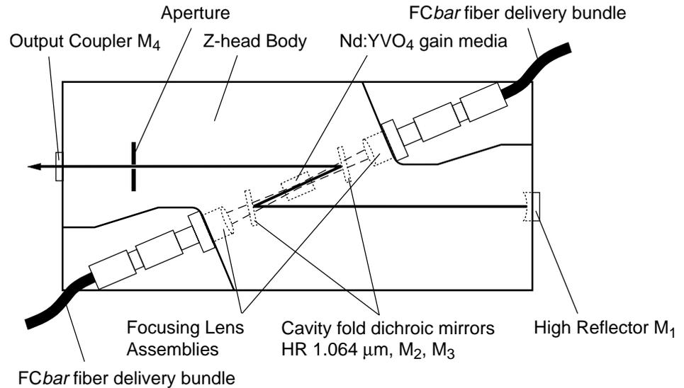
**Figure 3-10: The Z-Head (top view)**
