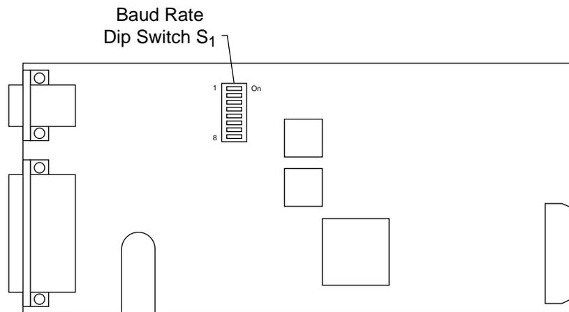
**Figure 6-3: Laser head pc board showing the location of baud rate dip switch S<sub>1</sub>.**
