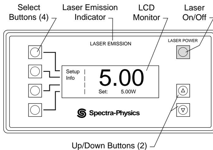
**Figure 4-3: The Millennia IR Control Module**
