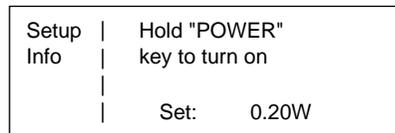
Press and hold in the LASER POWER button until the laser starts. When the button is pressed, the LASER EMISSION light flashes for a few seconds. Then, when laser emission occurs, it stops flashing and remains on, and the emission indicator on the laser head turns on to indicate radiation is present.
