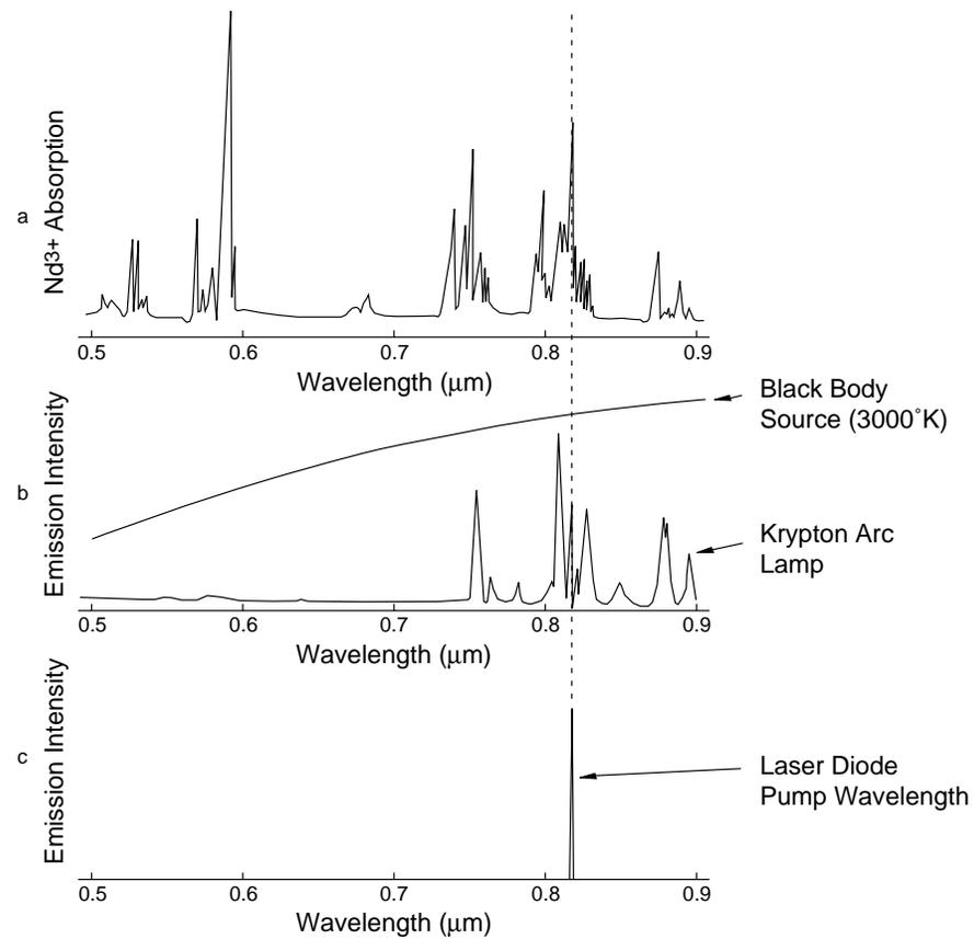
**Figure 3-5:  $\text{Nd}^{3+}$  absorption spectra compared to emission spectra of a Black Body Source (a), Krypton Arc Lamp (b) and a Laser Pump Diode (c).**
