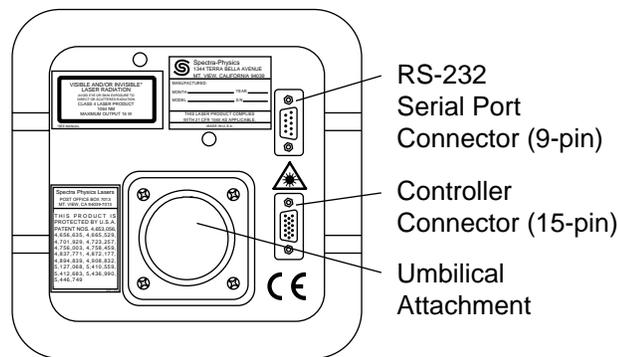
**Figure 4-2: The Millennia IR Laser Head Rear Panel**
