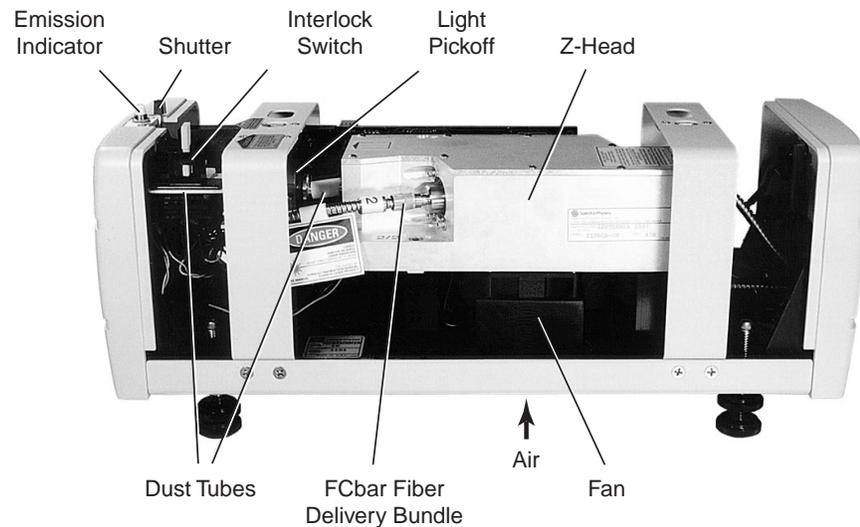
**Figure 3-8: The Millennium IR Laser Head**
