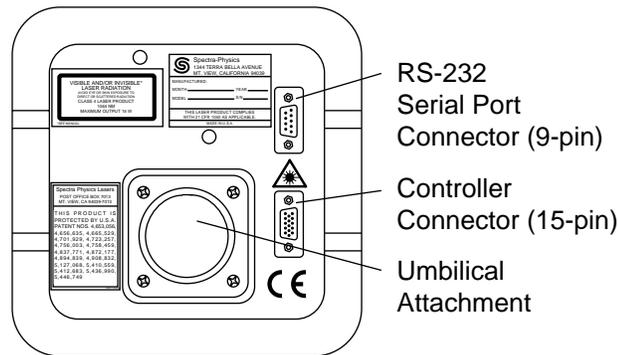
**Figure 5-1: The Millennia IR Laser Head Rear Panel**
