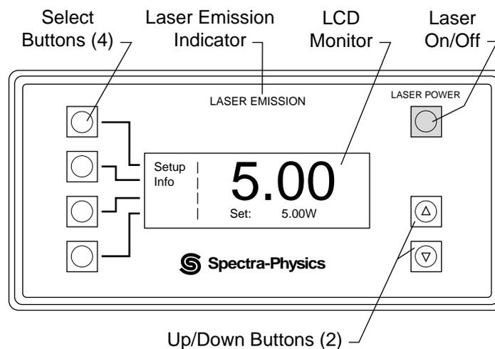
**Figure 6-1: The Millennium IR Controller Showing the Default Main Menu.**
