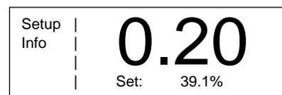
To change the power or current setpoint, simply press one of the up/down buttons. Note that when the buttons are held down, the setpoint numerical update pauses from time to time. This is normal. To change from power to current mode, or vice versa, use the Setup menu.
